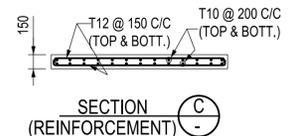
**SECTION (REINFORCEMENT) C-C**
