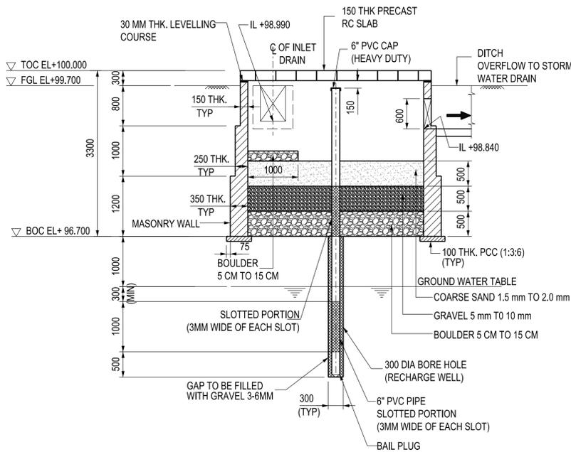
**SECTION (FORMWORK) F-F**
